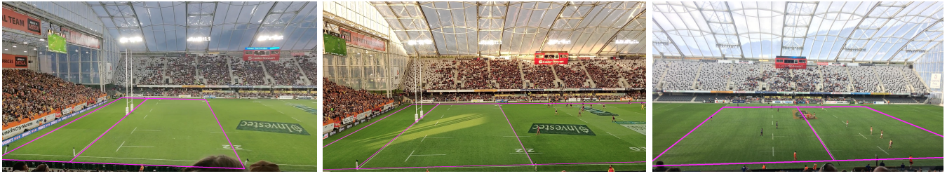
Fig. 7: Problems of our approach. Left) The bottom border of the field influencing our homography estimation. Middle) Error accumulated from detected outliers. Right) Homography estimation from the center being affected by a logo.
